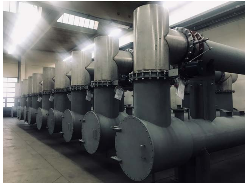
The picture shows the first 10 exhaust gas heat exchangers including mounted bypass before the dispatch at our premises in Gunzenhausen.
